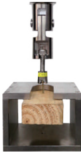
自攻牙拔出 / 拉穿 Withdrawal/Pull through
